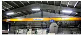
Reference: TIP-070 CRANE BRIDGE Year: 2006 Brand: AUSIO
